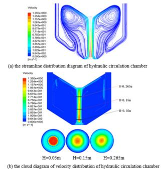
Figure 2: The CFD numerical simulation of hydraulic circulation chamber.
