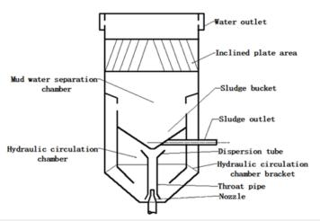
Figure 1: Schematic diagram of deep clarification device.
