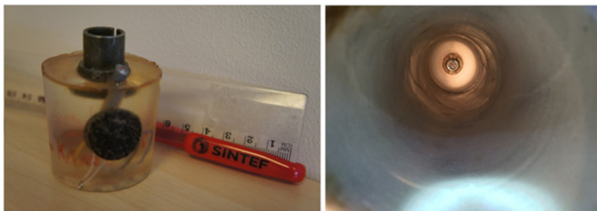
Figure 1: A long term door-stopper (left) and installation in a borehole (right).
