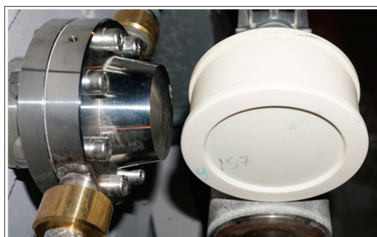
Figure 4: Container with sample opposite the accelerator target.
