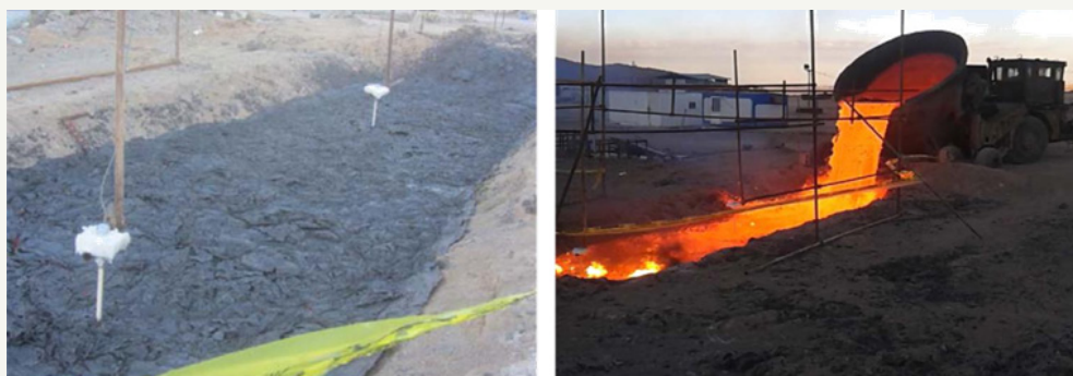
Figure 3: a) The location of the thermocouples in test, b) Slag loading in designed ditch.
