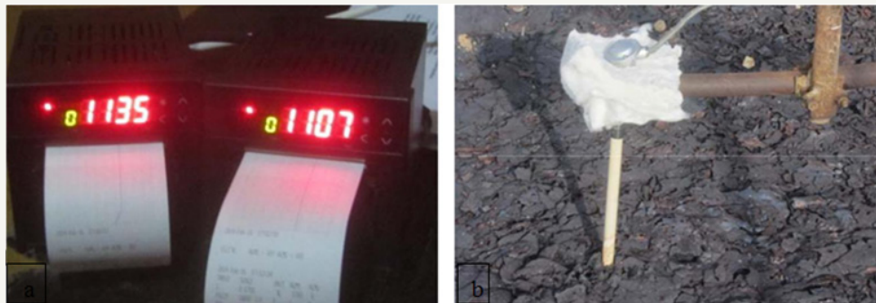
Figure 2: a) Temperature indicators used in experiment, b) The test thermocouples and coverage.
