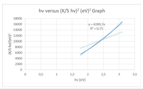
**Figure 2:**  $(K/S hv)^2$  versus hv graph of the cellulosic chromophores in tissue paper for the calculation of band gap energy for permitted indirect transitions n=2.
