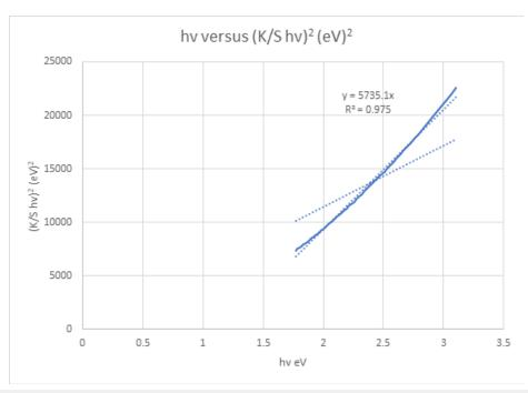
**Figure 8:**  $(K/S \text{ hv})^2$  versus hv graph of the cellulosic chromophores in copy A4 maestro paper for the calculation of band gap energy for permitted indirect transitions n=2.
