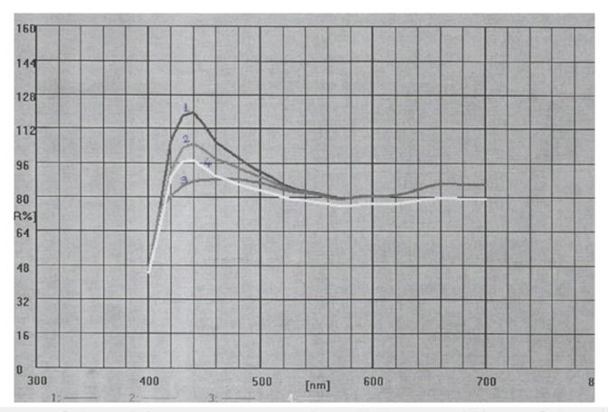
**Figure 3:** Reflection Graphs for copy paper A4 AXION sample: 1: D65 brightness, 2.ISO brightness (Reflection% C/2) 3.ISO brightness-UV (Reflection% with filter) 4. Opacity (Reflection% over black).
