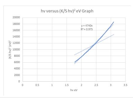
**Figure 6:**  $(K/S \text{ hv})^2$  versus hv graph of the cellulosic chromophores in velvet board for the calculation of band gap energy for permitted indirect transitions n=2.
