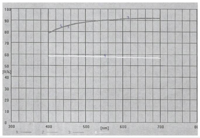
**Figure 1:** Reflection Graphs for tissue paper sample: 1: D65 brightness, 2.ISO brightness (Reflection% C/2) 3.ISO brightness-UV (Reflection% with filter) 4. Opacity (Reflection% over black).
