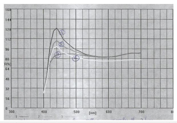
**Figure 7:** Reflection graphs for copy paper A4 maestro sample: 1: D65 Brightness, 2.ISO Brightness (Reflection% C/2) 3.ISO Brightness-UV (Reflection% with filter) 4. Opacity (Reflection% over black)
