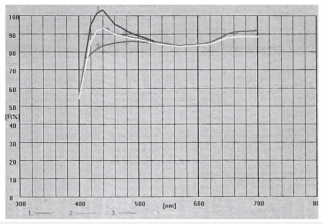
**Figure 5:** Reflection graphs for velvet board sample: 1: D65 Brightness, 2.ISO Brightness (Reflection% C/2) 3.ISO Brightness-UV (Reflection% with filter) 4. Opacity (Reflection% over black).
