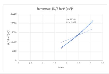
**Figure 4:**  $(K/S \text{ hv})^2$  versus hv graph of the cellulosic chromophores in copy paper A4 axion for the calculation of band gap energy for permitted indirect transitions n=2.
