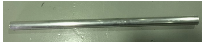
Figure 1: An aluminum pipe with (a 50 mm) outer diameter and (3 mm) thickness.
