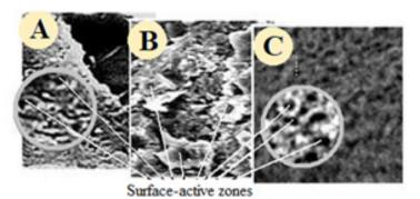
Figure 3: The fragments of the hydrated surface of cement grains of three-month (A, B) and 105-year (C) samples.
