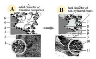
**Figure 1:** Diagram and general view of the initial (A) and final (B) states of the interacting cement system. 1-transition energy complexes; 2-surface clinker grain; 3-grain array; 4-active center; 5-dipole arch; 6-adsorption center; 7-molecule water; 8-residual active center; 9-hydrate product; 10-residual surface- active zones; 11-hydrated sheath
