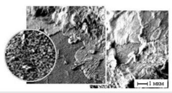
Figure 8: The structure of cement grains of 105 years of age.
