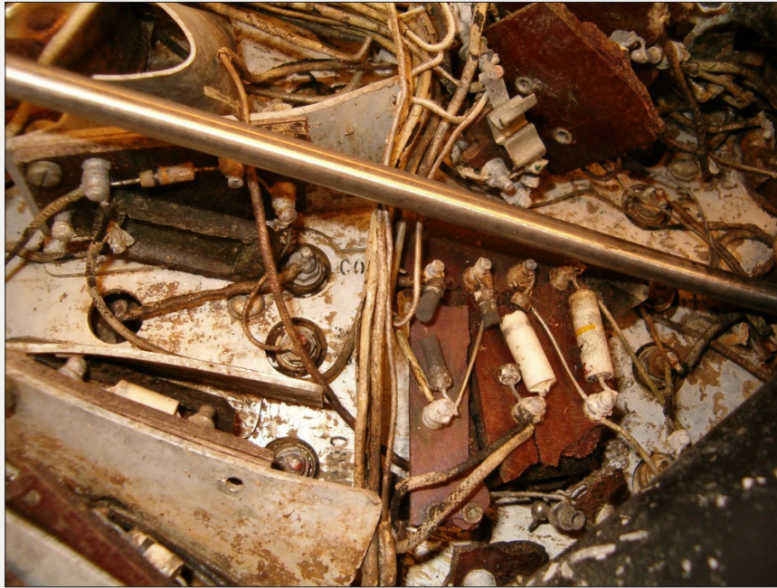
Figure 1: Mangled avionics from a B24 crash site during WW11 at the Gander, NL, Canada, airfield. An example of mass damage done by gravity.
